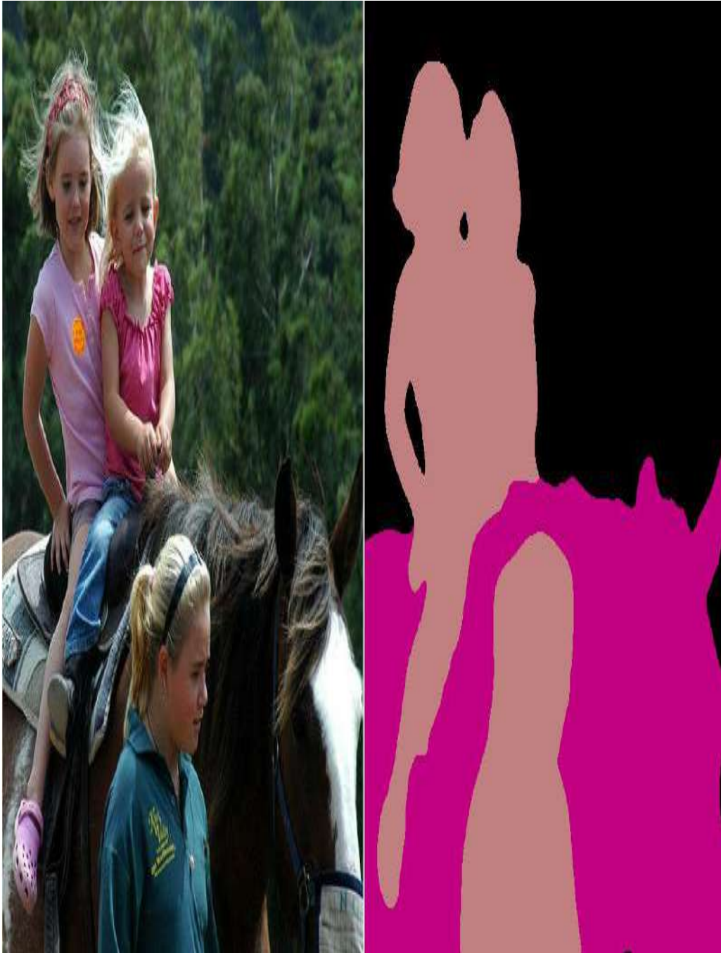
Figure 3.6 Example for Deep Lab Semantic Segmentation
